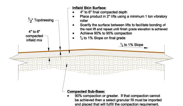
The compacted sub-grade should mirror finish grade to ensure that an even depth of material has been placed.
